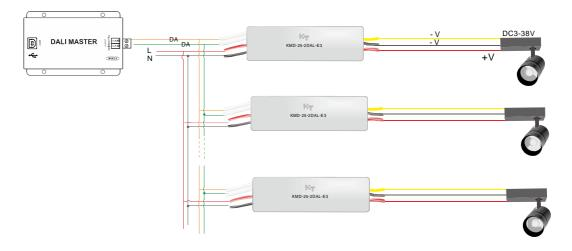
Dali Diammble Driver has synchronization function during the dimming process
