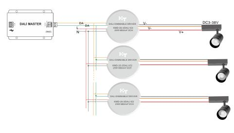
Dali Diammble Driver has synchronization function during the dimming process
